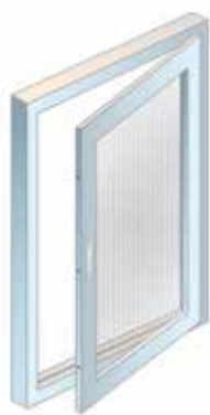
Hinged windows can open inward or outward.
